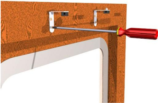
1. **Face fix:** Sola-Cure blinds are supplied with two L shaped brackets. The brackets are for use when face fixing only.
