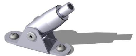
15. For additional tension, pull the wire through the base. Using long nosed pliers. It is possible to increase the tension in the wires by pulling the wire through further.
